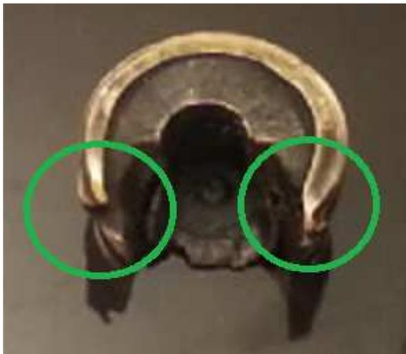
**2. The circular break of the case is clean but a deformation shows that the bottom part broke first (green circles), then around the case.**
