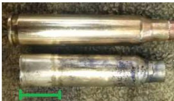
**3. You can see the stretch on the bottom of the case body before the break in the last 10-12 millimeters. (green area)**
