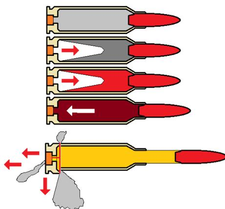
**10. A big flash-hole also can crate a "shaped charge" and breaking the powder**
