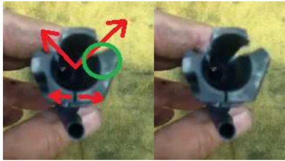
**5. The rear part of the bolt carrier is broken in the tiny part areas and the deformation is more important on the extractor side. (green circle)**
