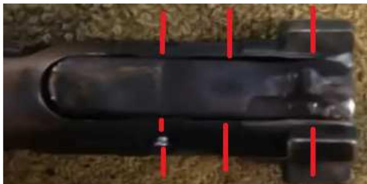
**7. The extractor lug doesn't seem so be damaged by a bad locking (right).
