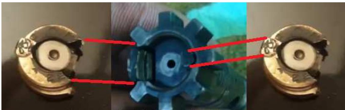
**4. The two significant traces left on the bottom of the case are the extractor zone and the ejector hole. But a closer look at the primer shows that it was overpressured but the fire pin mark is still clearly there. This is strange for a normal overpressure.**
